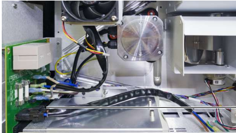
Power cable to AC board connector
