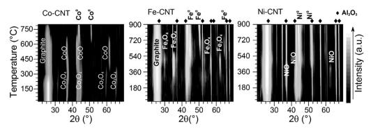
Fig. 2. Thermal transformation of CNT-supported metal nitrates. Contour maps of in-situ XRD in N2 atmosphere for M(NO3)x/CNT samples (Co(NO3)2; Fe(NO3)3 and Ni(NO3)2).
