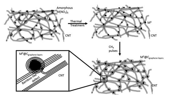
**Fig. 9.** Schematic representation of impregnation-reduction-decoration methodology to obtain metal-carbon hybrid materials (graphene-coated CNT-supported metal nanoparticles). Metal nitrates aqueous impregnation (a), in-situ thermal decomposition-reduction metal nitrates (b) and metallic nanoparticles decoration with some graphene layers by methane pulses decomposition (c), and corresponding zoomed in area (d).
