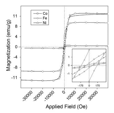
**Fig. 10.** Magnetization loops of M-hybrid material (graphene-coated CNT-supported Fe, Co and Ni nanoparticles) obtained by impregnation-reduction-decoration methodology.
