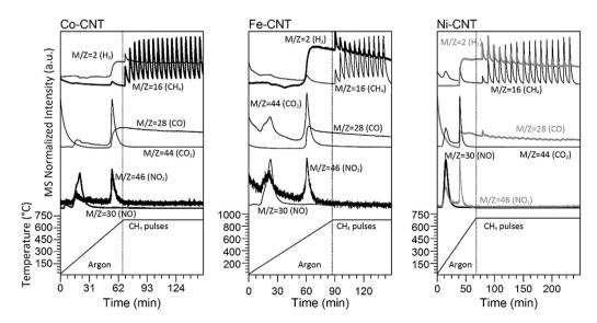
Fig. 3. MS profiles for M(NO<sub>3</sub>)<sub>x</sub>/CNT samples (Co(NO<sub>3</sub>)<sub>2</sub>; Fe(NO<sub>3</sub>)<sub>3</sub> and Ni(NO<sub>3</sub>)<sub>2</sub>). Thermal programmed in-situ decomposition of CNT-supported metal nitrates in Ar atmosphere and decomposition of CH<sub>4</sub> pulses during an isothermal step.
