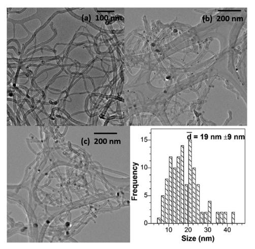
**Fig. 5.** TEM micrographs. Raw carbon nanotubes obtained during ethanol decomposition at 900 °C using LaFeO<sub>3</sub> as catalyst precursor (a). CNT after impregnation of Fe(NO<sub>3</sub>)<sub>3</sub> and in-situ decomposition (b); and after methane pulses decomposition at 900 °C (c). Iron metal particle size histogram (d).
