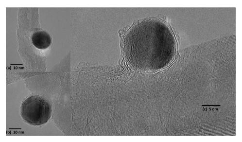
Fig. 8. HR-TEM micrographs for Ni-hybrid material (graphene-coated CNT-supported nickel nanoparticles) obtained by impregnation-reduction-decoration methodology at 700 °C as final temperature.
