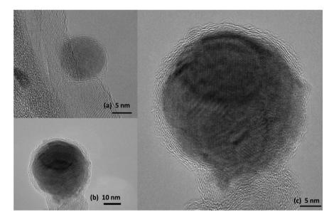
Fig. 7. HR-TEM micrographs for Co-hybrid material (graphene-coated CNT-supported cobalt nanoparticles) obtained by impregnation-reduction-decoration methodology at 700 °C as final temperature.
