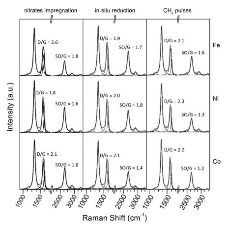
Fig. 4. Raman spectra for M-hybrid materials obtained by impregnation-reduction-decoration methodology. Spectra obtained after nitrates impregnation, thermal treatment under N<sub>2</sub> atmosphere (in-situ reduction) and methane pulses decomposition reaction, respectively.
