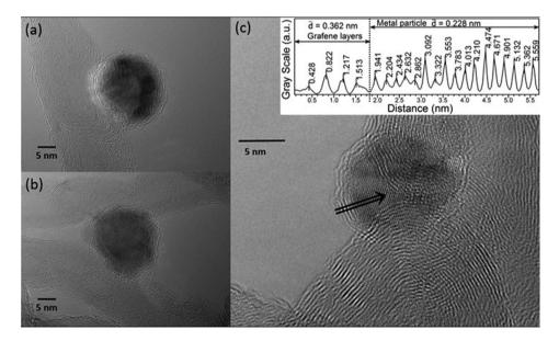
Fig. 6. HR-TEM micrographs for Fe-hybrid material (graphene-coated CNT-supported iron nanoparticles), obtained by impregnation-reduction-decoration methodology at 900 °C as final temperature.
