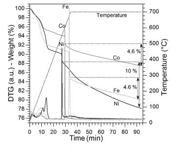
Fig. 1. Thermograms in  $N_{\rm 2}$  atmosphere for CNT impregnated with metal (Ni, Fe and Co) nitrates.
