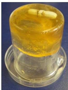
Figure 1. Self-crosslinked modified chitosan gel, produced by dissolving 6% (w/w) of the aldehyde-functionalized chitosan in distilled water under stirring (pH of the gel is ~5.5).
